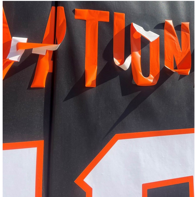
Following winter storm conditions (6°F): Competitive cast vinyl (top) vs. NextBond Premium Vinyl (bottom).
