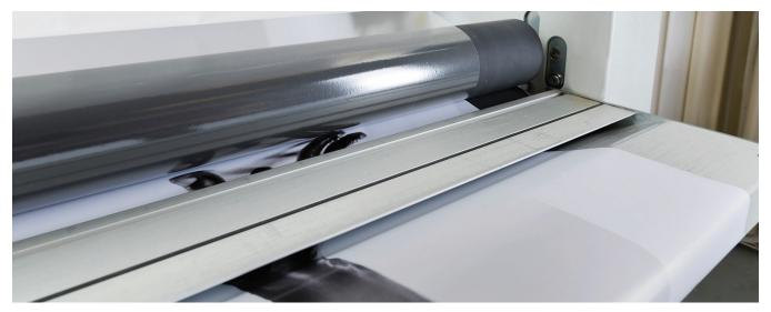
Eclypse<sup>™</sup> polymeric vinyl is an overlaminating film that protects against abrasion, chemicals and UV rays to extend the life of graphics.
